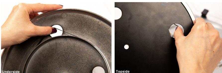
6. Gently lower the platter onto the central spindle of the base unit, ensuring that the elastic band is stretched over the drive shaft.
